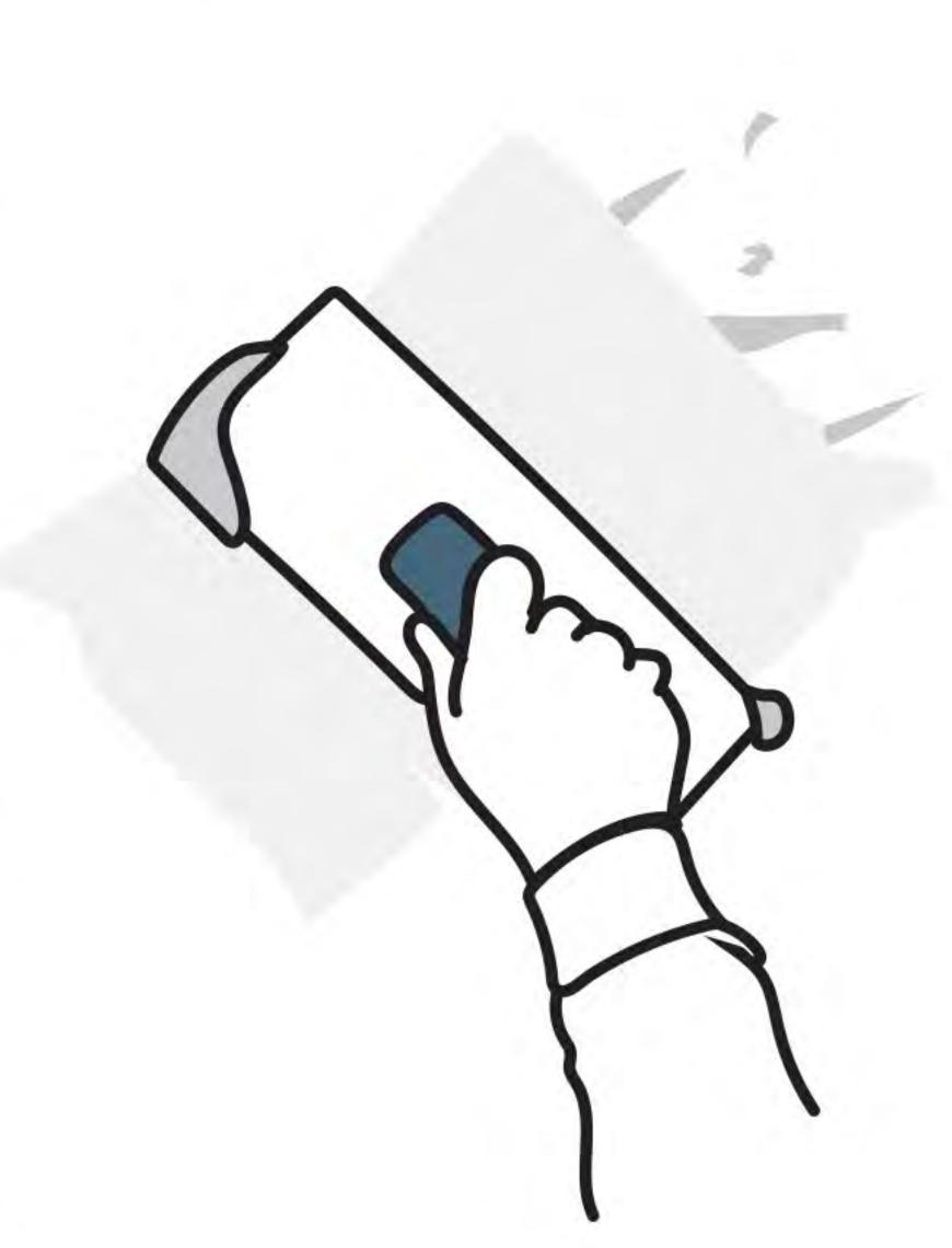
Loose, unstable material must be removed manually or mechani-Wall surfaces affected by mold or cally, and be repaired.
